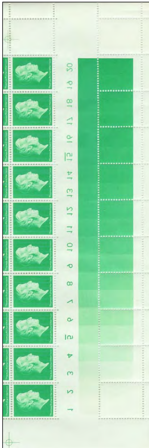
There is a diamond shaped phosphor area formed by the tips of the marginal cross hair. Also, the step wedge has a solid phosphor area in gutter.
