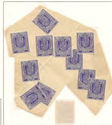
Test piece of eleven labels with two gripper marks and locating pin marks, as separate label shows. The 1/2 stamp affixing machine applied these labels.
