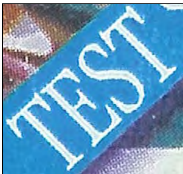
Normal litho with typical white spotty appearance, rosette pattern and a general loss of detail
