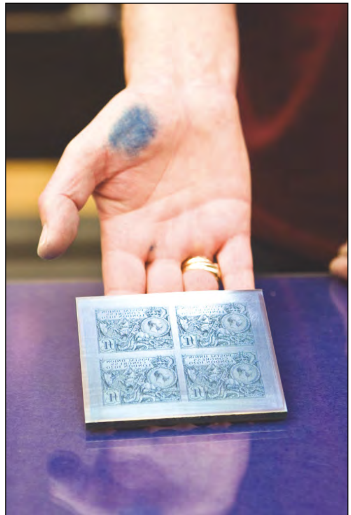
The inked plate comprising a block of four of the iconic and much loved £1 PUC design in a cleaned state and ready to be placed on to the printing press bed.
