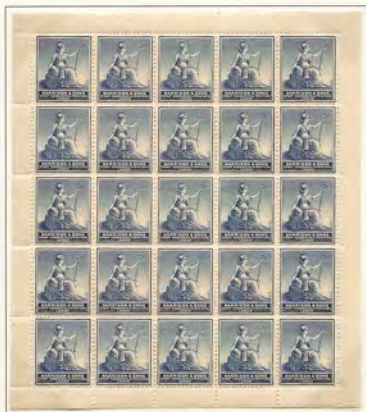
Sheet of 25 (5 x 5) labels using the letterpress process. Note that a single fine comb head was used, as shown by the non-alignment of the horizontal perforations at foot of each label.
