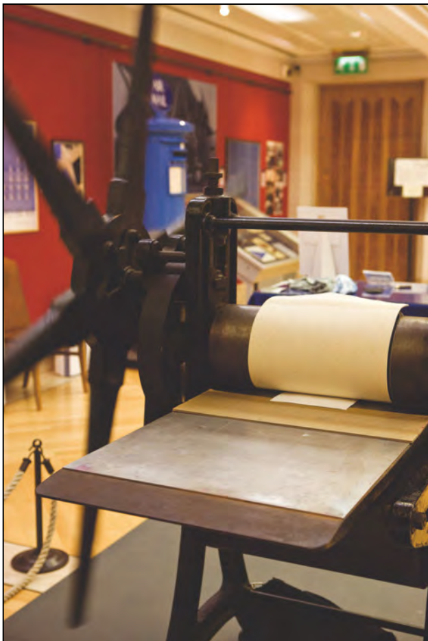
Paper placed on top of plate in readiness for printing.
