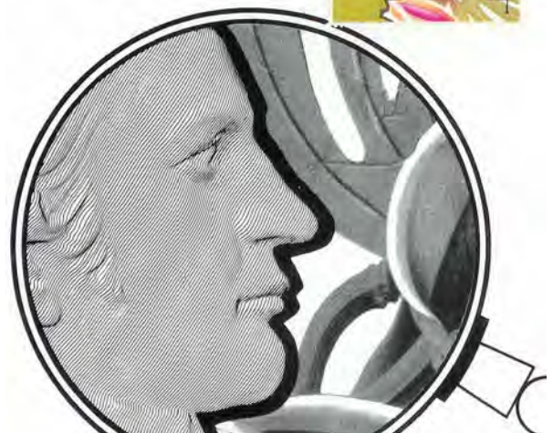
Enlarged area showing the detail achievable from this 90,000 dots to the square inch process.
