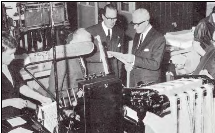
The Postmaster General, Edward Short, witnessing the embossing of the British Christmas stamps issue of 1966. Note the rolls of foil at bottom right of image. This gold foil working was applied by a Heidelberg platen press.
