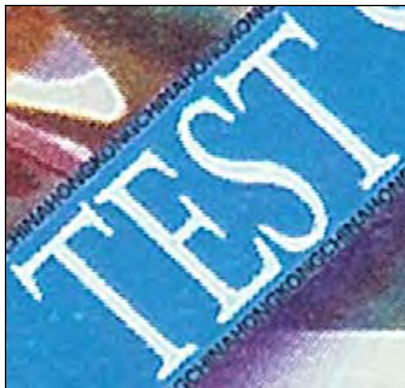
SuperLitho with micro-printing giving a superior image quality and greater detail, including micro-printing
