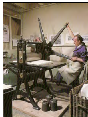
Applying pressure to plate.
