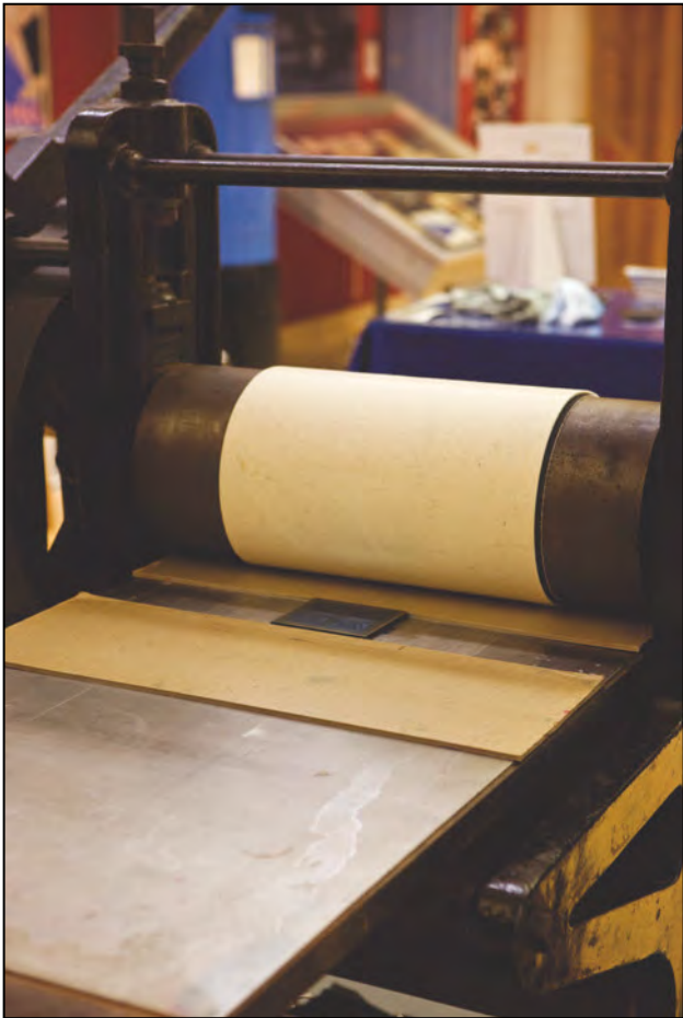
The printing plate on the flat bed of the press with hardboard at top and bottom to help keep it in position.
