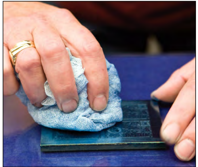
Removing excess ink from the surface of the printing plate by buffing it with a cleaning cloth.
