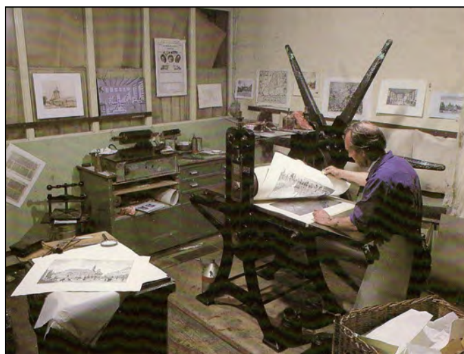
Slowly and carefully removing the printed sheet from the plate.
