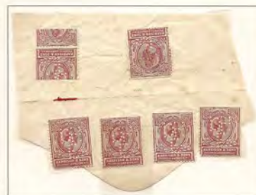
(right) Test piece of six labels from D H Evans (Beam) Poke affixing machine showing misplaced detachment cuts on one label.
